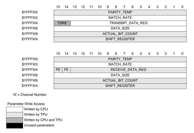
Figure 2 UART Function Parameter RAM Assignment
